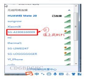
Enter the default IP address of Logger 1000/EyeM4 in the browser address bar after the device is connected: 11.11.11.1 to open the device management interface, the initial password is pw1111.
