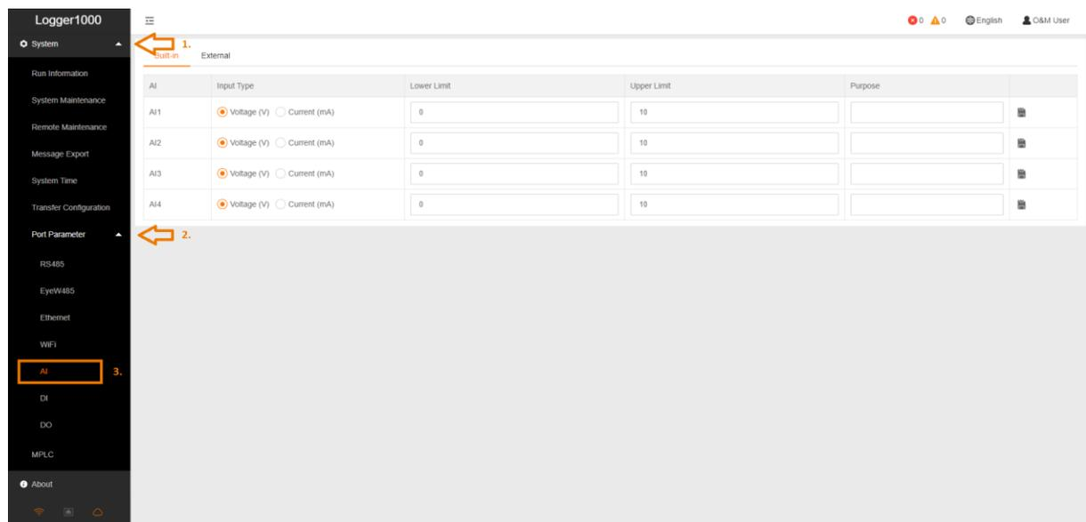
Now, you have the option, to configure four AI-ports, depending on which one you connected. Set **Voltage/Current** and corresponding values.
