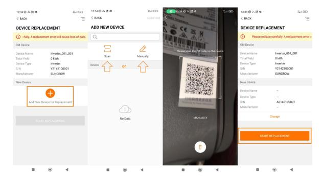
After the successful change of the inverter, the new device will be shown in the device overview.
