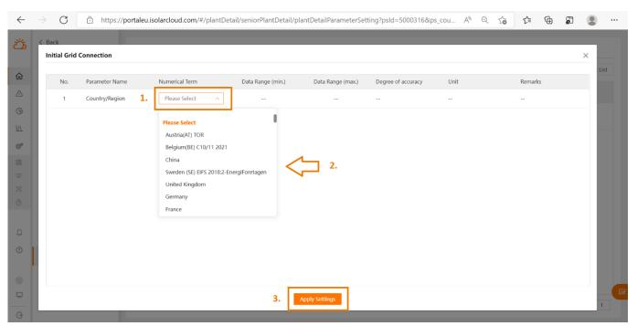
For some specific countries, it is required to perform additional manual settings. Follow the separate manual settings guideline. Enter the correct settings in the Common Parameters – Power control.
