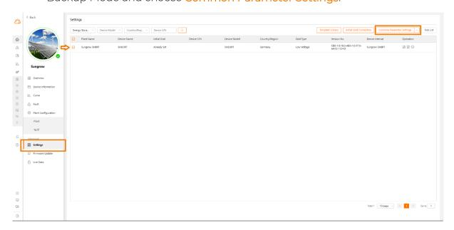
In the Common Parameter Settings, navigate to Power Control. Here you can enable Backup Mode and set the Reserved Battery SOC for Off-Grid operation. Apply Settings. Please be aware, that this Reserved Battery SOC cannot be used in daily operation as it is reserved for a power outage.
