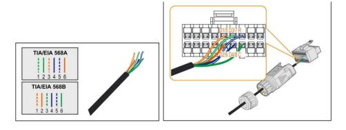
In particular, here is how the cable is wired to the communication connector of the hybrid.
