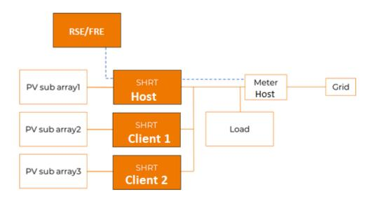
With Ripple Control Receiver it is possible to connect the 3-phase Hybrid with any other PV inverter in parallel. The signal wire, however, must be split in order to connect with both inverters (blue dotted line in the schematic below)
