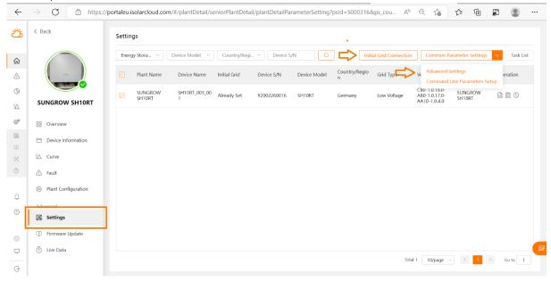
4. Make sure, you set Import (Total Purchased Energy)/Export (Total Feed-in Energy) Energy Adjustment, according to your previous screenshots. If the power generation compensation is not carried out, the power generation data on iSolarCloud will show anomaly.
