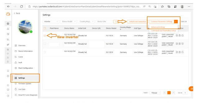
4. Make sure, you set Total Yield Adjustment, according to your previous screenshots. If the power generation compensation is not carried out, the power generation data on iSolarCloud will show anomaly.
